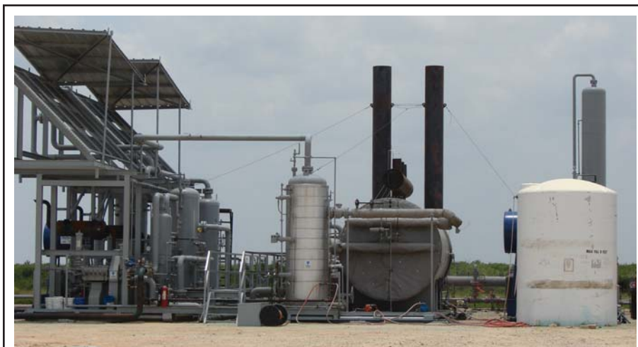
Valerus Compression Services' Enhanced Treating™ system is a compact, skid-mounted gas treating unit that utilizes special contactors to enhance contact and absorption rates. No outside power is needed because the system runs on a natural gas-powered generator, and it uses 40 percent less fuel than conventional plants.
